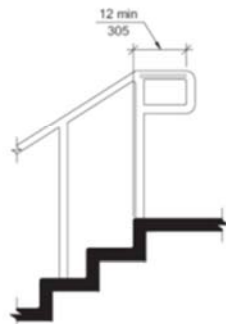
FIG. 505.10.2 TOP HANDRAIL EXTENSIONS AT STAIRS
